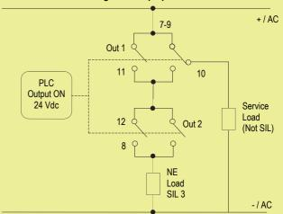
Contacts 7-11 and 8-12: the SIL 3 Safety Function is met when the relay is energized, contacts are open, load is de-energized.
