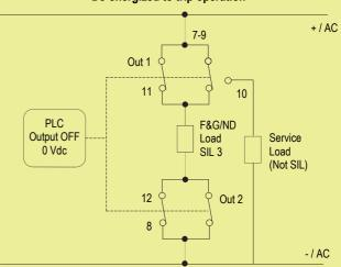
**Contacts 7-11 and 8-12:** the SIL 3 Safety Function is met when the relay is de-energized, contacts are closed, load is energized.
