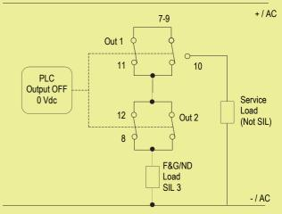
**Contacts 7-11 and 8-12:** the SIL 3 Safety Function is met when the relay is de-energized, contacts are closed, load is energized.
