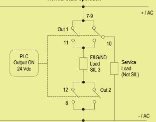
Contacts 7-11 and 8-12: in normal operation the relay is energized, contacts are open, load is de-energized.
