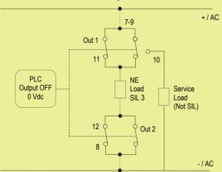
Contacts 7-11 and 8-12: in normal operation the relay is de-energized, contacts are closed, load is energized.
